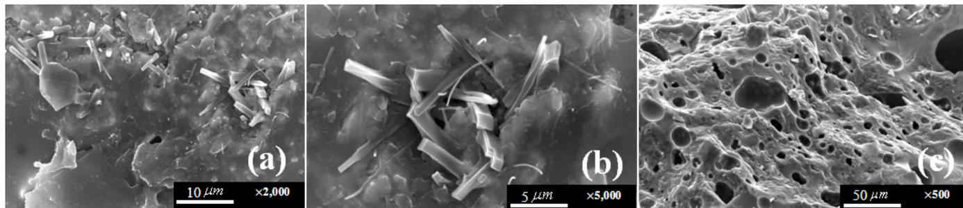
**Figure 2** SEM micrograph of 850°C sintered sample at top surface (a)2,000 and (b)5,000 magnification and at inside sample (c)500 magnification
