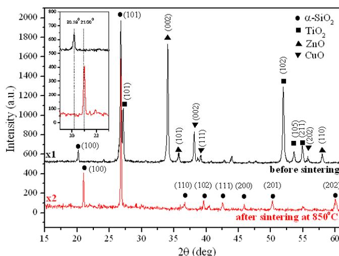
**Figure 1** XRD pattern of the powder and the  $850^\circ \text{C}$ -sintered samples.
